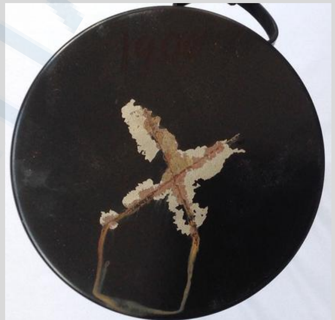
Corrosion after 1800 Hrs of salt spray chamber test.
