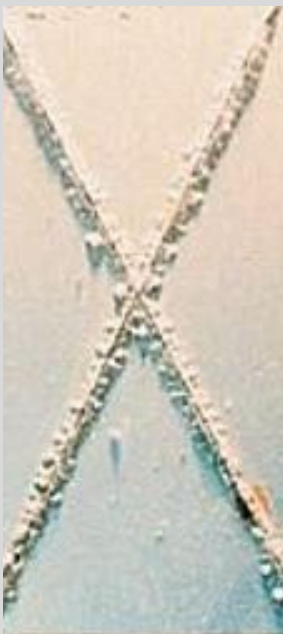
Corrosion after 1100 Hrs
