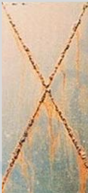
Corrosion after 1450 Hrs
