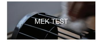
To assess the adhesion of EcoAtex to metal, we conducted the **MEK test**. In this test, **a cotton ball is soaked in a methyl ethyl ketone (MEK) solution and rubbed 40 times over the coated specimen**. The test is considered successful if no paint transfers from the part to the cotton ball.
